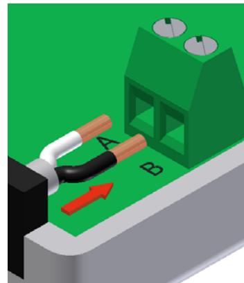
Connect the wires into the green terminal block Make sure you do not reverse the polarity.
